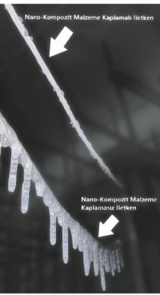
The "Deflection and Leakage Preventing Nano-Composite Material for MV Lines" project, developed under the leadership of MEDAŞ in collaboration with Dicle Elektrik Dağıtım A.Ş. and Ketronik A.S., seeks to provide innovative solutions to the challenges faced in electricity distribution lines. This project offers an effective solution to problems such as conductor breaks and pole collapses caused by icing and severe weather conditions, particularly in winter.
